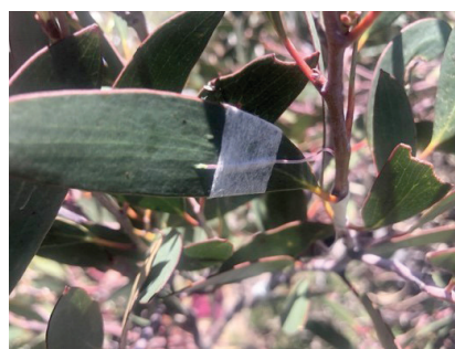
Thermocouple wire inserted into a Eucalyptus pauciflora leaf and secured with tape in Kosciuszko National Park.
