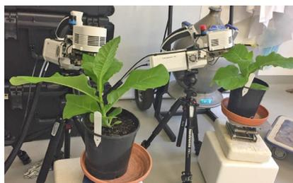
Measuring gas exchange using LiCor 6800 machines
