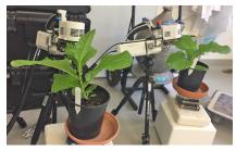
Measuring gas exchange using LiCor 6800 machines
